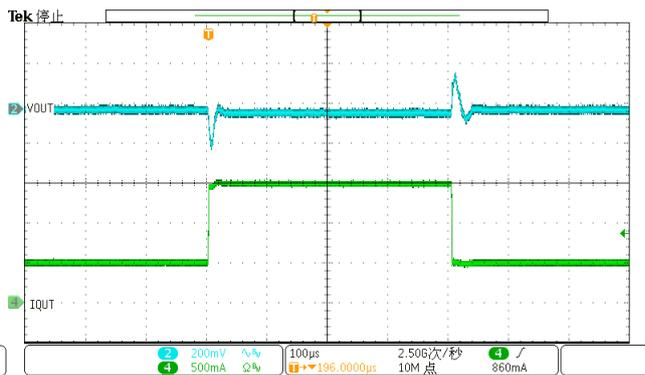
Load Transient;  $V_{IN}=28V, V_{EN}=5V, V_{OUT}=5V, I_{OUT}=0.5A-1.5A$
