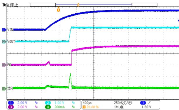
Start up from VIN, VIN= 3.3V, VOUT=1.2V, IOUT=0A
