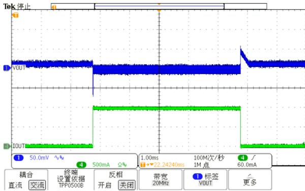
Load Transient,  $V_{IN}=3.3V, V_{OUT}=1.8V; I_{OUT}=1mA\sim 1A$
