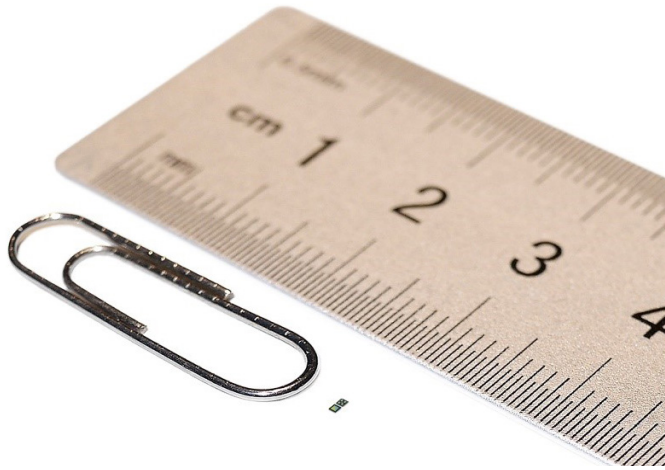
Figure 4—OMNIVISION holds the Guinness World Record for the world's smallest image sensor, pictured here.
