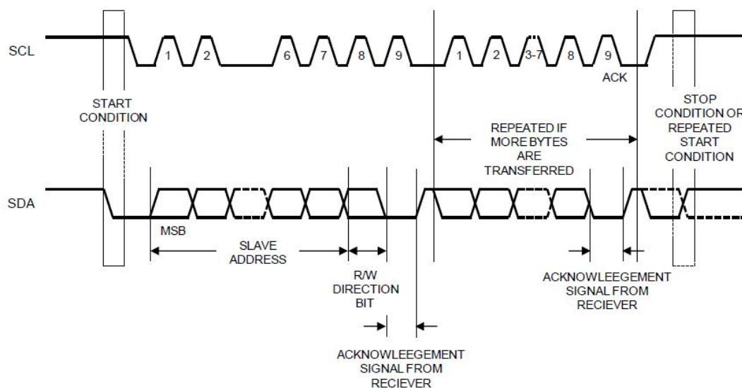
**Figure 3. Data Transfer on I<sup>2</sup>C Serial Bus**
