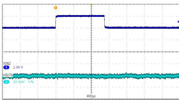
**Power Supply Ripple Rejection (PSRR)**
