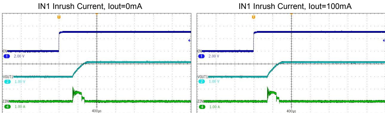
VIN2 Inrush Current (LDO3/4 Cout=1uF, LDO5/6 Cout=2.2uF, LDO7 Cout=1uF, Total Cout=7.4uF)
