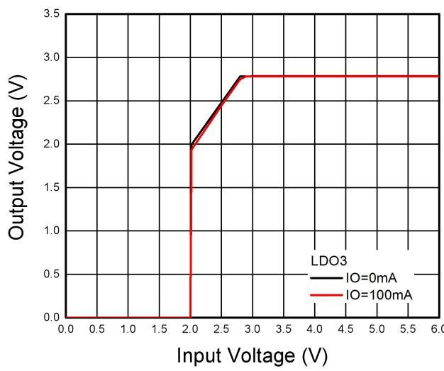
**Output Voltage vs. Input Voltage 2**
