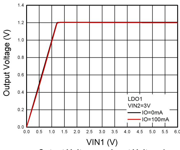
**Output Voltage vs. Input Voltage1**
