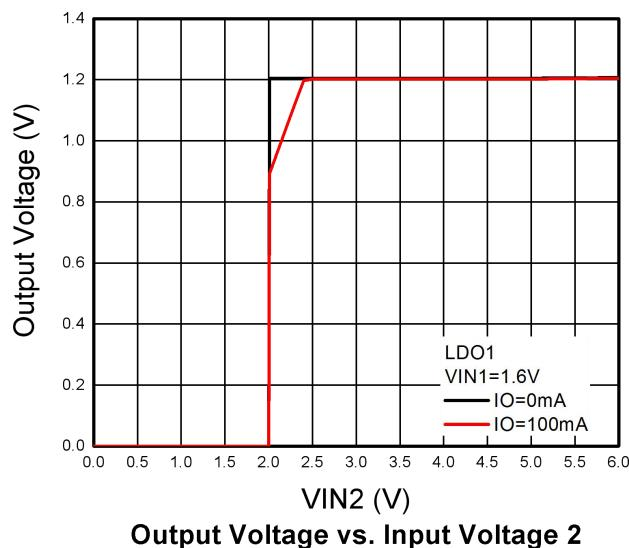
**Output Voltage vs. Input Voltage 2**
