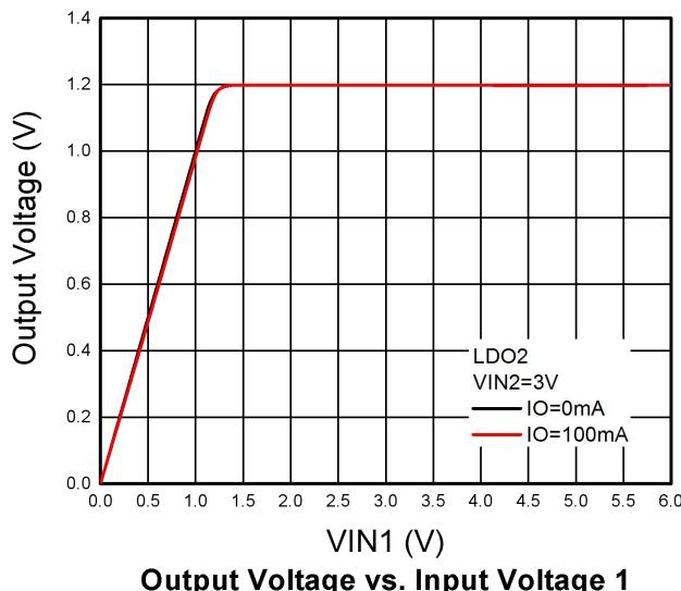
**Output Voltage vs. Input Voltage 1**
