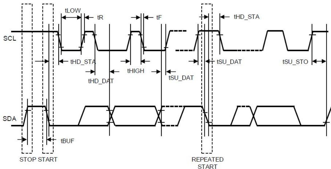
**Figure 2. I<sup>2</sup>C Mode Timing Diagram**
