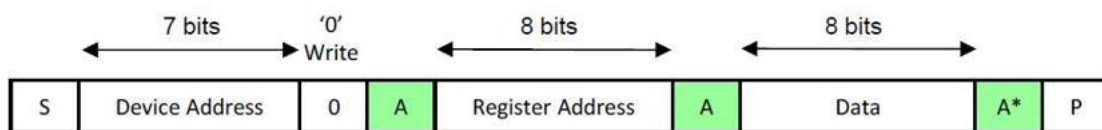
I 2 C Write – Slave Receiver Mode
